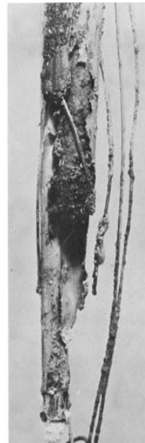
Bottom section of damaged fuel bundle
