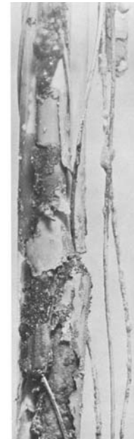
Mid-section of damaged fuel bundle
